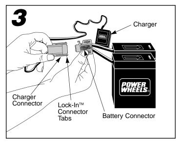
Squeeze the Lock-In<sup>™</sup> connector tabs on the charger connector and plug it into the battery connector.
